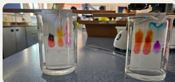
Ink colours separated into vibrant patterns during chromatography experiments.
